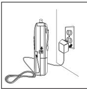
Use the included AC Adapter/Charger to power the **BC60XLT** from an AC source. The AC Adapter/
